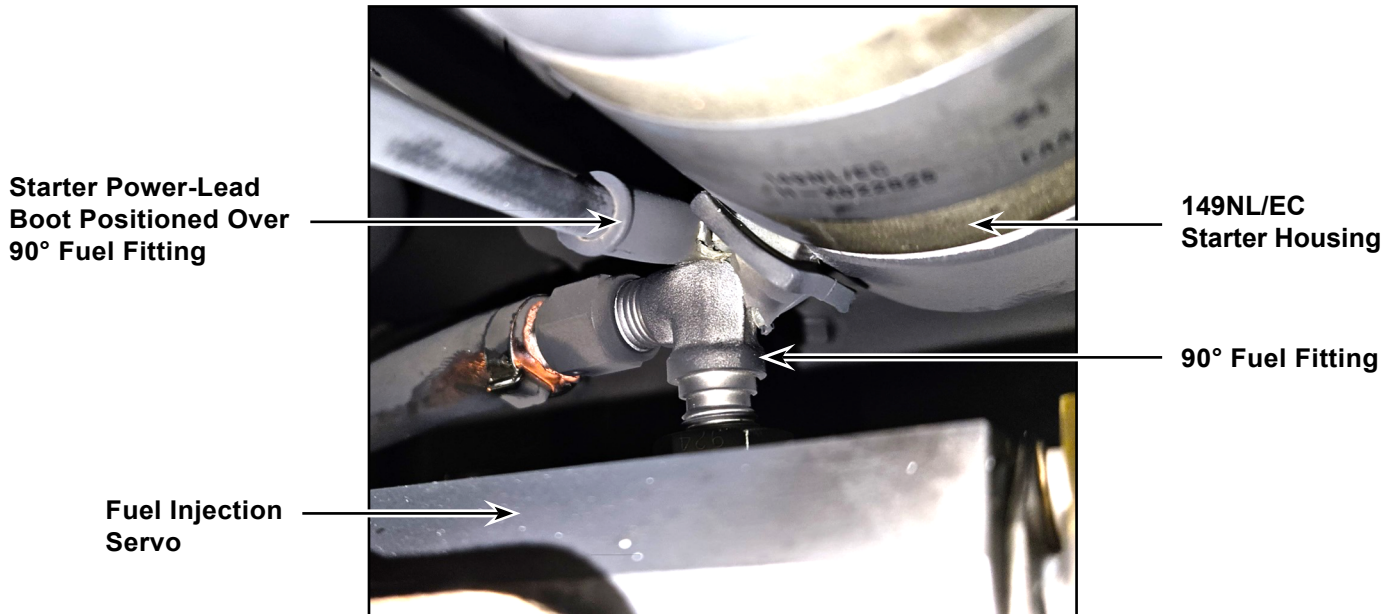
Figure-1 - Improper Starter Installation
