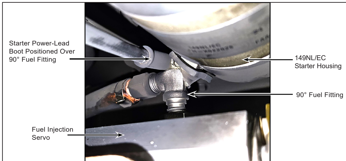
Figure 6.1 – Improper Starter Installation
